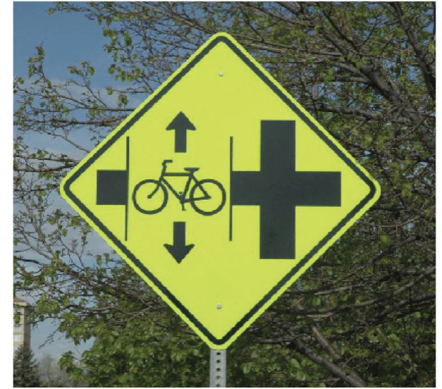
Sidepath Advisory Signs. Top: Variation of the MUTCD's Railroad Advance Warning Sign, modified as a sidepath advisory. This sign should be used on both sides of a road with sidepaths. This installation is on Speer Boulevard in Denver, advising of the parallel Cherry Creek Trail. Florida DOT advises a similar sign. Below: Trail crossing advisory sign on an intersecting side street, installed on Clayton Road in suburban Saint Louis.
