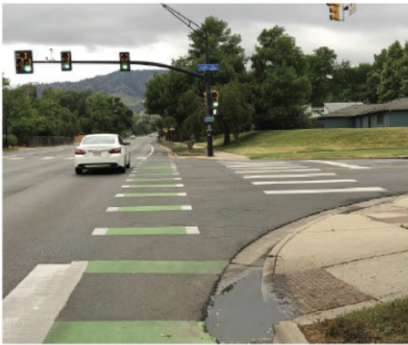
Use of color to increase visibility for sidepaths and bike lanes.
